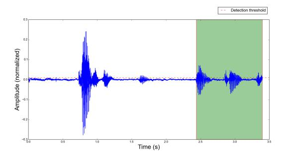
Finally it is almost always interesting to limit the length of detected audio activities. In any case, one does not want a too long audio event such as an alarm or a drill to hog the detector. For illustration purposes, we set the maximum duration to 0.4 second for this detector, so an audio activity is delivered as soon as it reaches 0.4 second:
